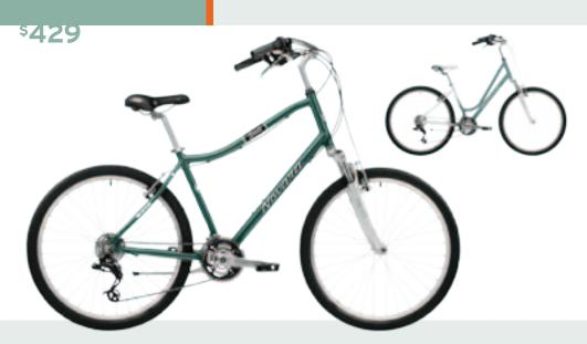
**OUR NEW BEST FOOT FORWARD TECHNOLOGY** We've moved the crank forward and slackened the angle of the seat tube, so riders can put their feet down easily without compromising pedaling efficiency.
