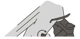
To return the battery to the bike, make sure the key is still turned to the unlocked position (clockwise). Line up and set the battery on the shelf at the bottom first, then click the top back into place. Last, turn the key back counterclockwise to lock the battery into place.
