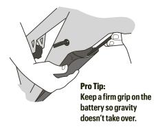
Unlock and remove the battery with your key to charge inside during extreme temps.
