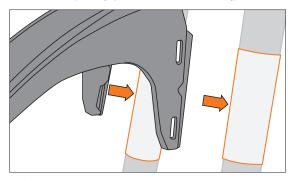
2. Thread the velcro strap with the rubberized side to the frame. Always retighten the straps before the ride!
