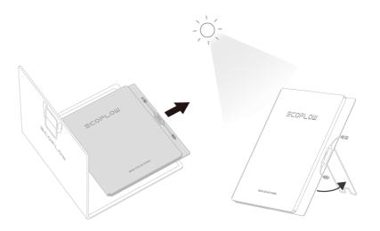
As shown in the picture, it's recommended to unfold the bracket first before unfolding the panel.
