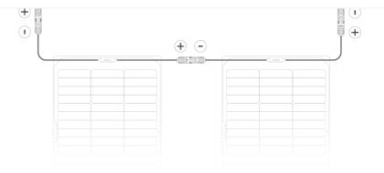
To wire **in parallel**, connect all positive ends of the panels' output cables to a solar parallel connection cable, and do the same for the negative ends. Then, connect the solar to XT60i charging cable to the solar parallel connection cables. When connecting, refer to the instruction images to avoid misconnecting the male and female connectors of the parallel connection cables.
