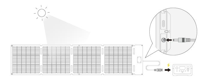
Connect the DC5521 port of the panel to your device's solar input port (XT60) using the provided DC5521 to XT60i cable.
