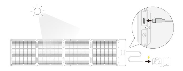
Prepare a Type-C charging cable, and use it to connect the panel's Type-C port to your device.
