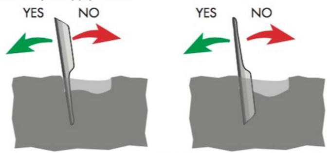
The Deuce's strength comes from its curved 'U' shape. Levering and scooping by bracing against the bottom of the 'U' shape, the Deuce® is amazingly strong and tough. BUT if you pry by bracing the Deuce against the open side of the 'U', it's much less strong.
