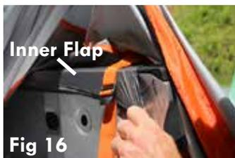
**12-**Adjust all straps a final time. Make sure that the inner side flap seams run along the top outer edges of the bed rails (Fig 16).
