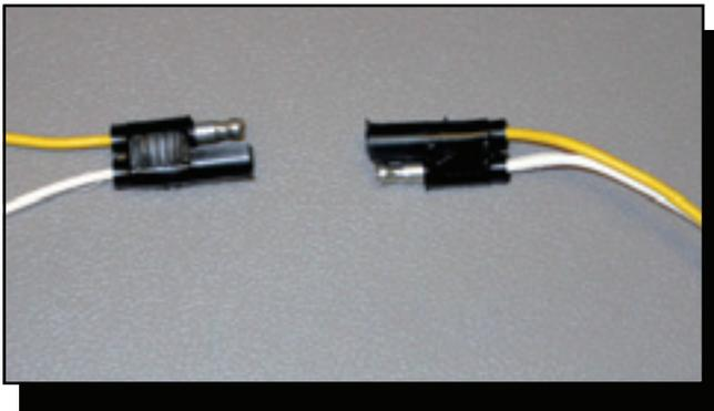
Figure 11—Polarized connectors could prevent improper electrical connections.
