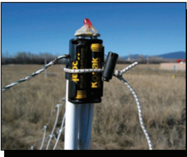
Figure 5—LEDs (light-emitting diodes) attached to two sides of a portable electric mesh fence can warn campers or animals before they touch or run into the fence.
