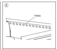
Be sure to keep the stack of firewood below the holes inside the main unit. If the firewood is stacked higher than the holes, it will continue to generate smoke
