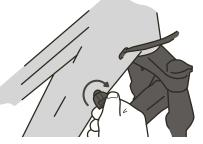
To return the battery to the bike, make sure the key is still turned to the unlocked position (clockwise). Line up and set the battery on the shelf at the bottom first, then click the top back into place. Last, turn the key back counterclockwise to lock the battery into place.
