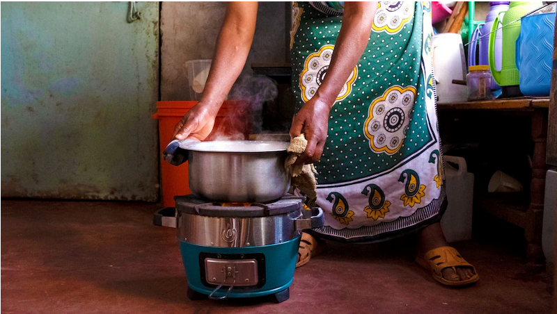
High-efficiency cookstove that cuts fuel consumption in half compared to a regular charcoal stove
