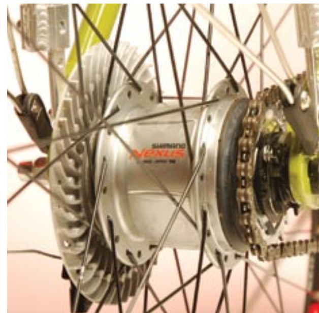
Low-maintenance internal gearing.
